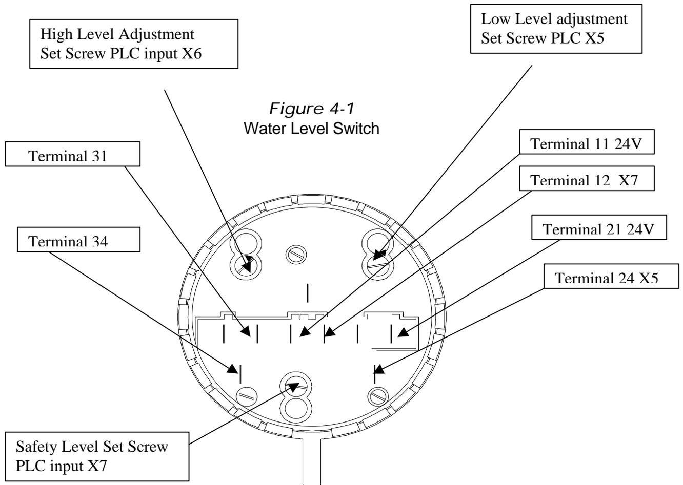
Water level adjustment instructions: to lower level settings, rotate set screw counter-clockwise; to raise level settings, rotate set screw clockwise. PLC inputs X5 and X6 will illuminate when water level is attained. X7 will illuminate when water level drains below a safe level for extraction step. Machine will not extract unless X7 is illuminated.
