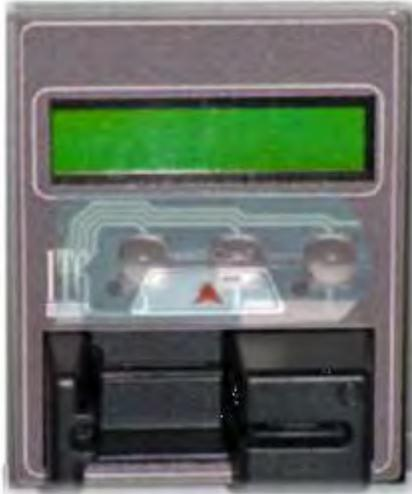
(1) The buttons are located below the screen and above the card reader, as shown in the picture of the CAD to the left. There are three buttons, one on the left, one in the center, and one on the right. The buttons are also shown in the graphic on the diagnostic menu below, labeled “DONE” on the left, “SELECT” in the middle, and “NEXT” on the right.
