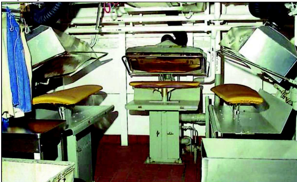
Figure 2-12 — Laundry press single-operator station.
