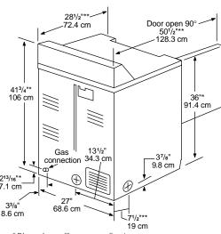
\* Dimensions will vary according to adjustment of leveling legs; add 1/2" min.
