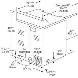
\* Includes 3/4" for hinge on back of dryer. \*\* Dimensions will vary according to adjustment of leveling legs; add 1/2" min
